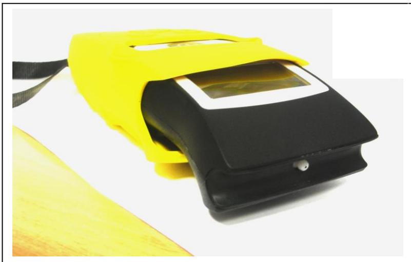
To replace the batteries the skin should be removed from the instrument to allow access to the battery compartment.
