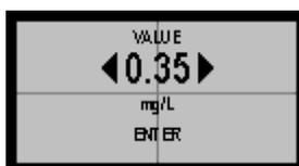
Use **DB** and **UB** to change the displayed number to agree with the known alcohol standard (after making any allowance for altitude for a dry-gas); then press **AB** to **ENTER**.
