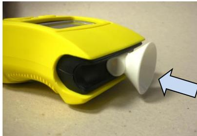
This test is an indicative test and will only give a pass or fail result, it should only be used to determine if there is alcohol present in the exhaled breath from a subject. For more accurate testing it is recommended that a mouthpiece test is carried out.
