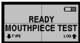
The display shows the battery status and the type of test that it is ready to take.
